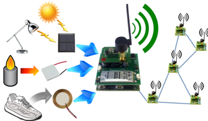
Figure 5: PowWow WSN Platform with Energy Harvesting
