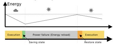
Checkpoints ensure task execution progresses [RBB<sup>+</sup>]. Spreading task processing over phases with energy allows complex computing on architectures without a battery, only a super-capacity with very low charge [SAS<sup>+</sup>]. These systems have multiple energy harvesters [PW] controlled by an efficient energy planner.
